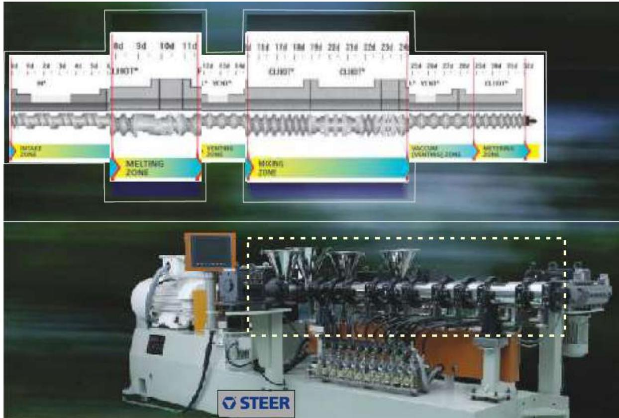
Melting and Mixing are the two giant (meteoric) steps that take place inside the Extruder Processing Zone (EPZ) of a co-rotating twin-screw extruder. Enhancement of melting and mixing is the key to achieve some extraordinary results. What remained an impossible task so far in most of the difficult applications has now become manageable, thanks to this new technology, invented by the author.
