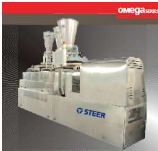
STEER'S GENERATION NEXT CO-ROTATING TWIN-SCREW EXTRUDERS
