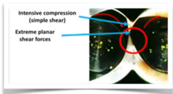
lobes at the tips of the barrel apexes. Material passing through this environment will experience a significant amount of shear energy input and high temperatures from frictional heating. If the solids content within the resin is high, as is experienced in masterbatch production, additional abrading of the mica can occur from particle-to-particle friction.
