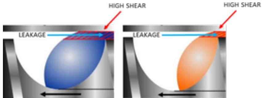
Perhaps *more damaging to effect pigment is the shearing that can occur when plastic containing the pigment "leaks" back into the trailing screw channel.*
