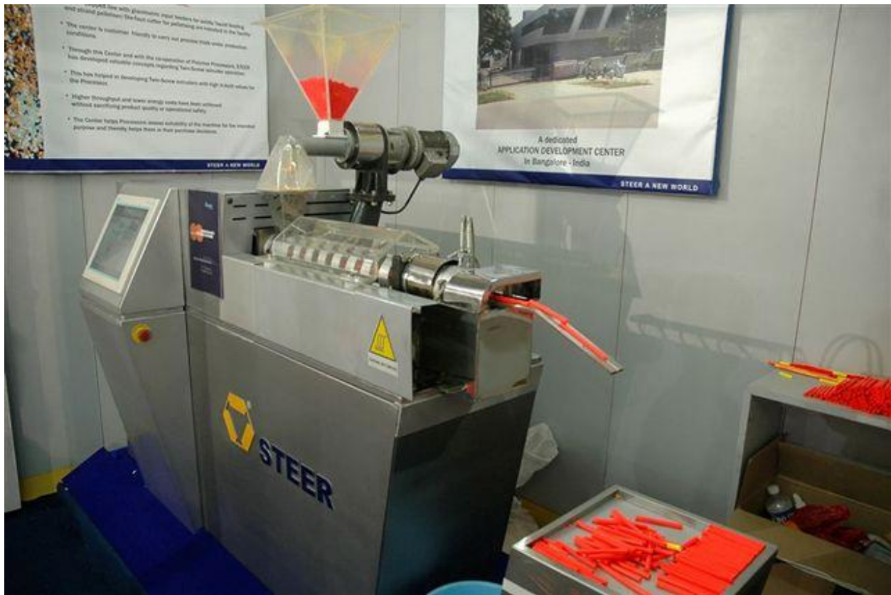
Figure 8. Glass walled transparent Extruder
