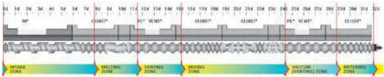
Figure 3: Process Zone in a Co-rotating twin-screw extruder
