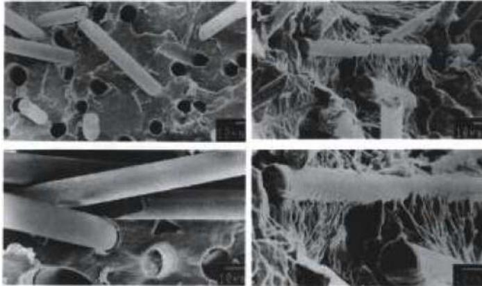
Figure 1: SEM Pictures of Glass Fiber Wetting & Coupling
